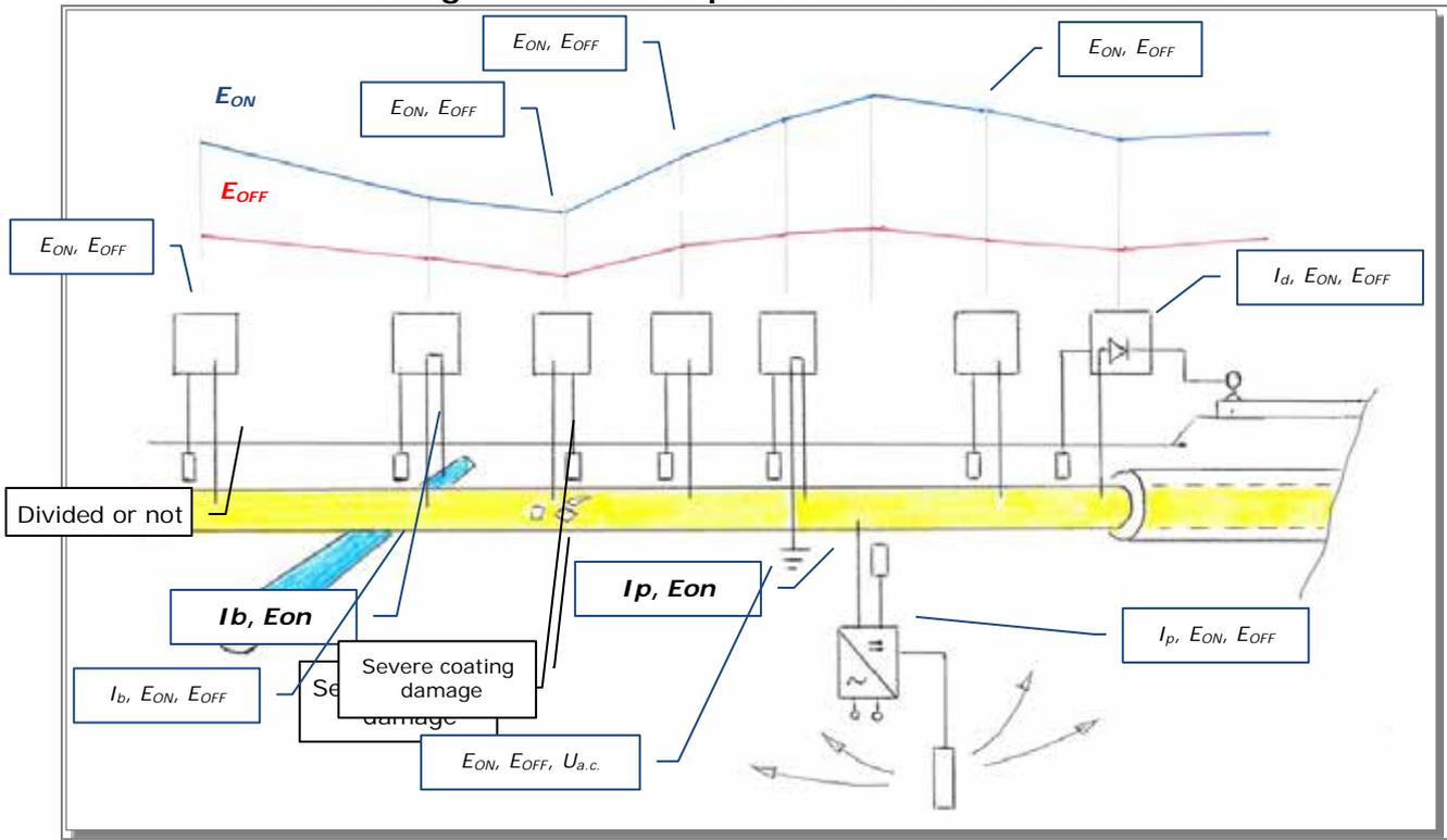
**Figure 3 – Remote monitoring of CP effectiveness (detailed and comprehensive assessment): monitoring of functional operation + all test stations**
