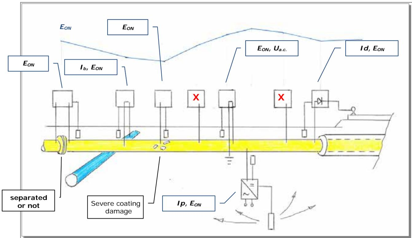
**Figure 2 – Remote monitoring of CP effectiveness (general assessment): monitoring of functional operation + selected test stations**
